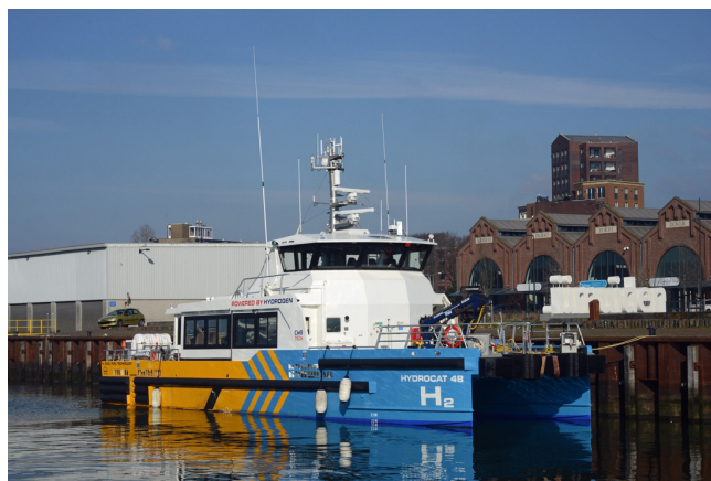
The Hydrocat 48, the world's first dual-fuel hydrogen- and marine gas oil-powered offshore wind farm service vessel. It mostly runs on fossil "grey hydrogen" due to a lack of available green hydrogen, but its owner Vestas intends to switch this ship and others to run on green hydrogen if/when that fuel becomes more widely available.
